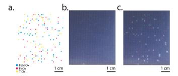
**Figure 1.** Proof-of-concept bubble evolution results from three different electrocatalysts randomly populated on an FTO coated glass. (a) The sample distributions of three electrocatalyst compositions are shown as cyan (FeNiO<sub>x</sub>), magenta (FeO<sub>x</sub>), and yellow (TiO<sub>x</sub>). (b) A snapshot of the bubble evolution video at t = 0. c). A snapshot of the bubble evolution video at t = 25 s showing registration with the FeNiO<sub>x</sub> catalysts.
