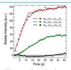
**Figure 3.** Bubble intensity as a function of time for an active catalyst (red), a moderate catalyst (green) and an inactive catalyst (black), where the solid lines were fitted data with two distinctive slopes.
