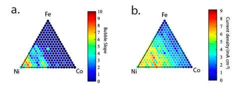
Figure 4. (Ni–Fe–Co)O<sub>x</sub> pseudoternary compositional maps of catalyst Figures of merit: (a) The bubble evolution slope from the parallel bubble screening and (b) the current density at 750 mv vs Ag/AgCl from serial scanning droplet cell measurement.
