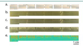
**Figure 2.** (a) Optical images of a pseudoternary material library,  $(Ni-Fe-Co)O_{x^*}$  (b) Snap-shots of the bubble evolution before applying the electrochemical potential and after application of the electrochemical potential (750 mV vs Ag/AgCl) at 0 s (c) and 20 s (d). (e). Background subtracted bubble image at 20 s. Note that the bright pixels in panel b are an artifact from the substrate (not bubbles) and are effectively removed by the background subtraction, as shown in panel e.
