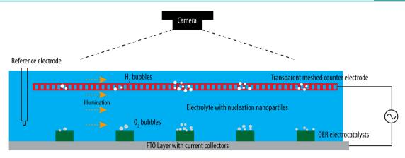
Figure 6. Cross-sectional schematic illustration of the bubble screening setup, where the green rectangles represent the testing material library, the red bars represent the transparent meshed counter electrode.
